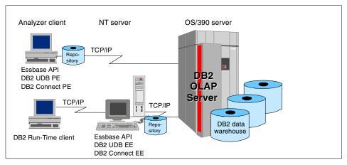
Figure 103. Analyzer 2- and 3-tier connections to DB2 OLAP Server for OS/390
