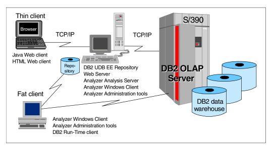
Figure 132. Three-tier DB2 Olap Server Analyzer configuration
