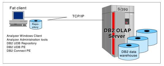
Figure 133. Two-tier DB2 OLAP Server Analyzer configuration
