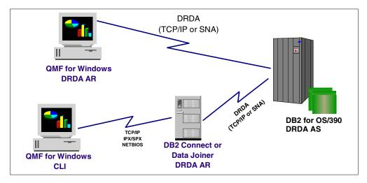
Figure 35. QMF for Windows connections to a DB2 for OS/390 data warehouse
