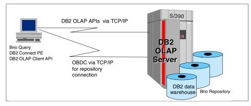
Figure 75. BRIOQuery to DB2 OLAP Server 2-tier connection
