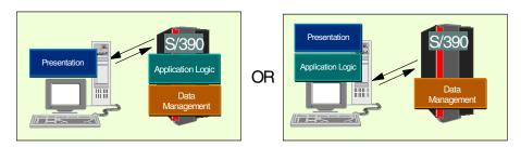
Figure 5. Three-tier logical application with two-tier physical implementation
