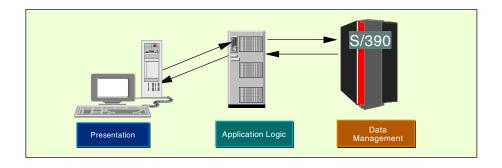
Figure 6. Three-tier logical application with three-tier physical implementation
