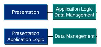
Figure 3. Logical two-tier application architecture
