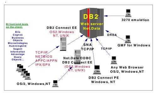
Figure 7. BI connectivity to the DB2 data warehouse on OS/390
