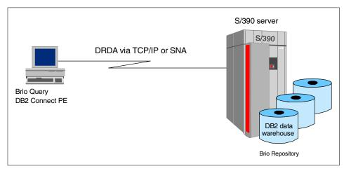
Figure 65. BrioQuery to DB2 data warehouse 2-tier connection
